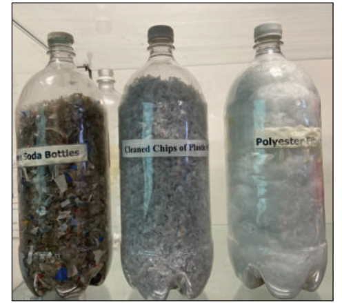
On display at the Prince George's County Materials Recycling Facility are some end products of the process, including plastic chips and polyester filler.
