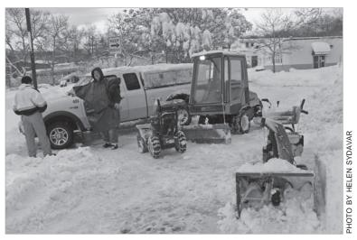
No, this is not a coffee break - Fredy Herrera (left) and Les Stampfer (right) are waiting for parts. The vibrations from hours of constant use had caused the retaining nuts to fall off the wheels of the snowblowers. Each wheel has two retaining nuts but one snow blower was missing both nuts from one side, so nothing was holding the wheel on. The other snowblower was missing one nut from each wheel. Notice that the snowblowers also have snow chains for traction.
