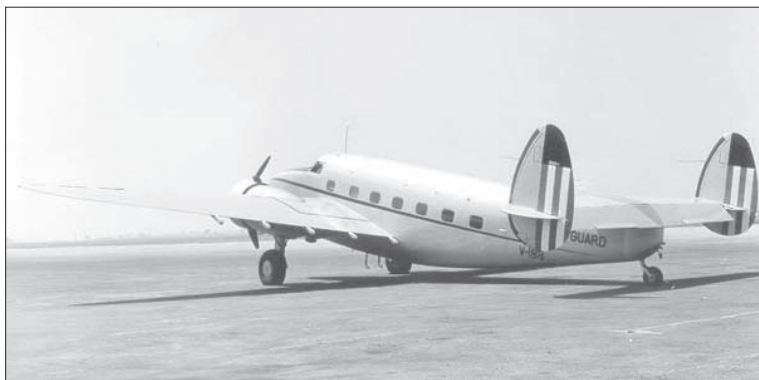
The Lockheed Lodestar R-50 is the type of plane that Lt. William Needham was flying when he crashed in 1945 at the Beltsville Airfield. It is similar in appearance to a DC-3.
