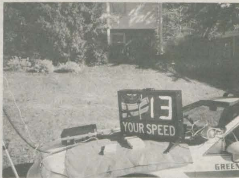
Speed display sign placed on top of Greenbelt squad car hood used to monitor speed on streets. Lakeside residents will use radar attached to this sign to monitor speed on their streets.
