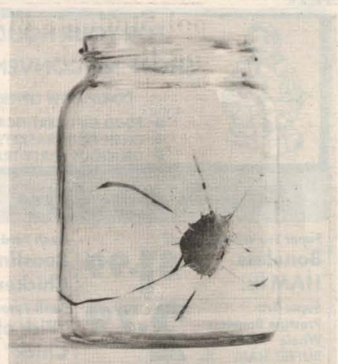
Recycling Problem — This glass container shows the effect of contamination. For recycling to succeed, recycled material must meet quality standards similar to the raw ingredients being replaced.
