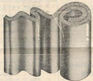
To slow heat loss through walls, ceilings and floors, you can choose among several thermal insulation materials, each in different forms. Glass fiber, mineral wool and cellulose fiber are available as loose fill...or sandwiched between layers of paper, in blankets, or in rectangular "batts."
