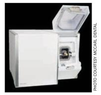
This Glidewell milling machine produces high fidelity crowns and implants made from zirconia
