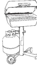
Each year, about 600 fires/explosions nationally occur with gas grills resulting in injuries to dozens of people. Propane gas is highly flammable. The new safety standard for propane gas tanks requires that an "over-fill prevention device" be installed in new gas tanks. The new propane gas tanks have valve handles with three "lobes" (prongs) while older tanks have valve handles with five prongs. People with older propane gas tanks should trade them in for the new, safer tanks.
