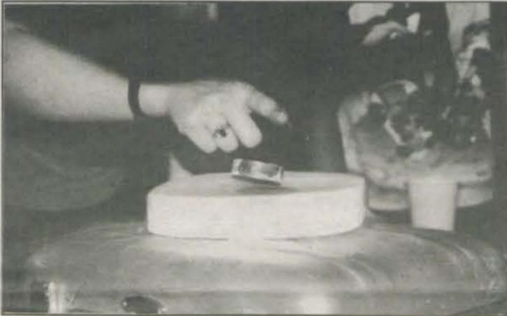
Dr. Peter Chen of NASA's Goddard Space Flight Center demonstrated super conductivity by floating super conductivity material above a magnet, both cooled by liquid nitrogen.
